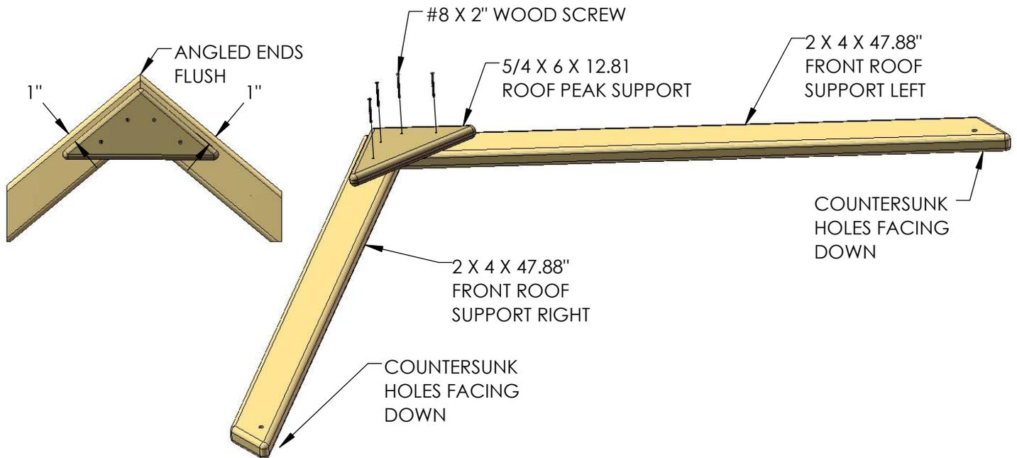
4: FLIP OVER THE ROOF SUPPORT ASSEMBLY, COUNTERSUNK HOLES SHOULD BE FACING UP. PLACE THE FRONT PLASTIC ARCH ON TOP OF THE ROOF SUPPORTS MAKING SURE THE TOP EDGES OF THE FRONT PLASTIC ARCH ARE FLUSH TO THE TOP EDGES OF THE ROOF SUPPORT ASSEMBLY ON BOTH SIDES. FASTEN USING #8 X 1-1/4" WOOD SCREWS. THE FINAL ASSEMBLY SHOULD MEASURE 69-7/8" AT THE BOTTOM.
