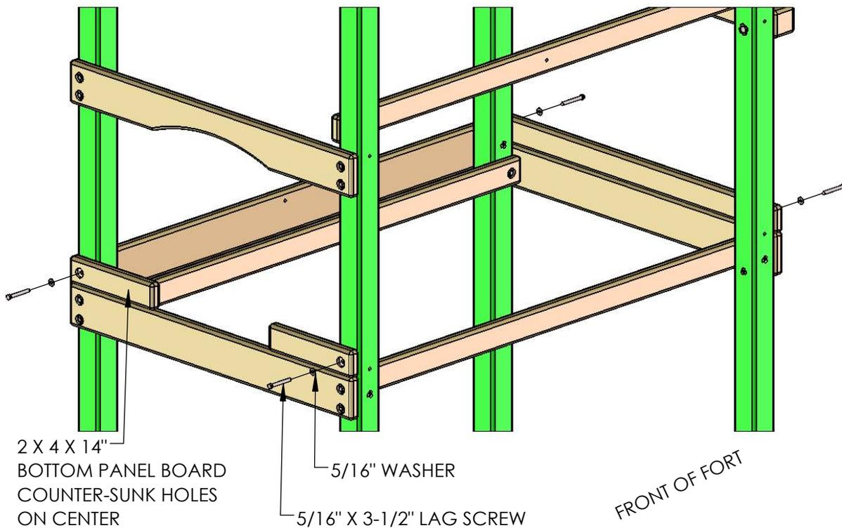
2: PLACE THE 2 X 4 X 47-1/2" BOTTOM PANEL BOARD (HOLES OFFSET UP) ON TOP OF THE 2 X 6 PANEL BOARD AND FASTEN TO THE CORNER POSTS WITH 5/16" X 3-1/2" LAG SCREWS AND 5/16" WASHERS.
