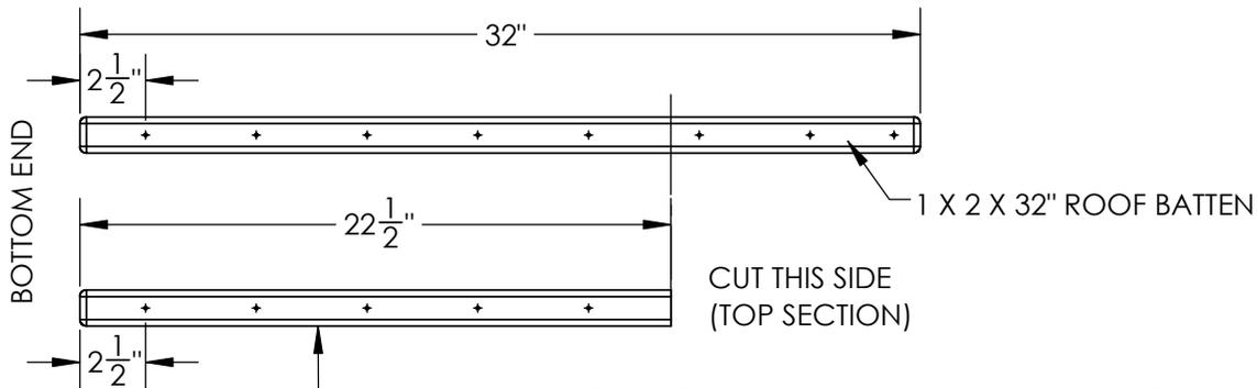
3: ONCE THE ROOF BATTEN HAS BEEN CUT TO 22-1/2", PLACE IT AGAINST THE REAR ROOF PANEL. THE UNFINISHED END (TOP END) MUST BE POINTING TOWARDS THE ROOF PEAK, AND THE BOTTOM END MUST BE FLUSH TO THE BOTTOM EDGE OF THE ROOF FINISHER. INSERT 1-1/4" WOOD SCREWS THROUGH THE PRE-DRILLED HOLES ALONG THE BATTEN.
