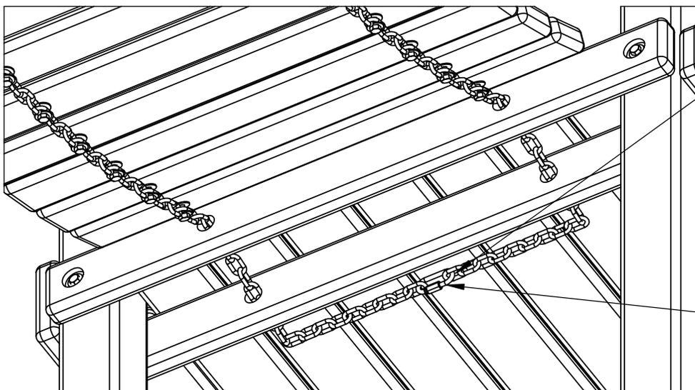
NOTE: TO ACHIEVE THE CORRECT GAP YOU MAY NOT BE CONNECTING THE END LINK OF EACH CHAIN. FOR EXAMPLE YOU MAY HAVE TO CONNECT THE SECOND, THIRD OR FORTH LINKS TOGETHER.
