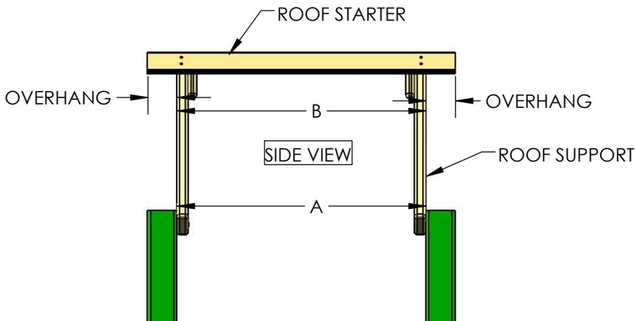
BEFORE INSTALLING THE ROOF STARTERS MAKE SURE DIMENSIONS A AND B MATCH. ALSO MAINTAIN THE SAME OVERHANG OF THE ROOF STARTERS ON EACH SIDE OF THE ROOF SUPPORTS.
